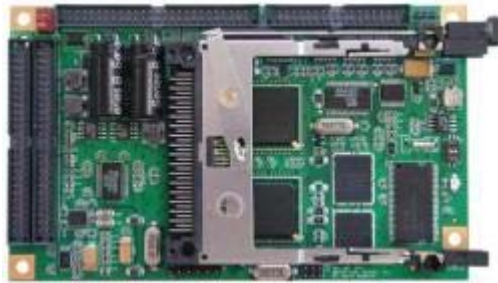
An ADS BitsyPlus serves as the embedded computer (Click for larger view)
